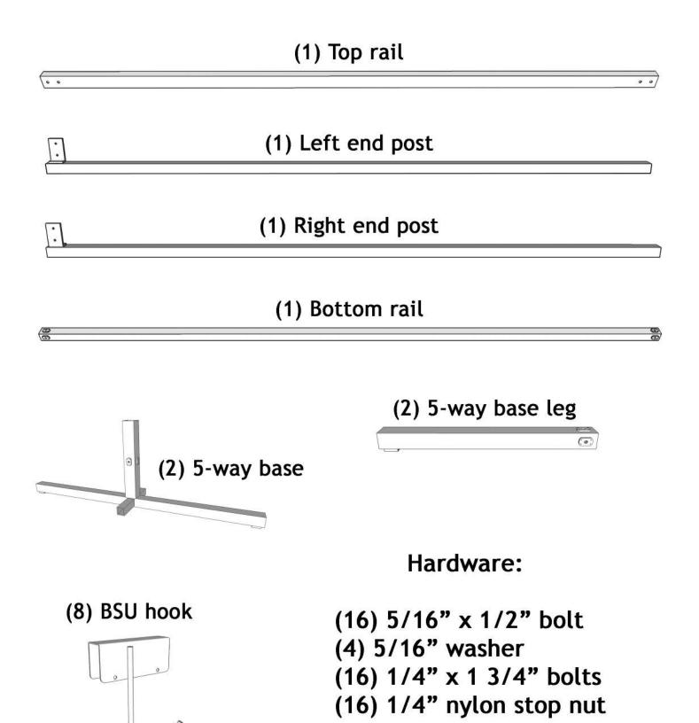
bases and the 5-way base legs. Slide the legs over the ears on the 5 way bases as shown and secure tighten using 5/16" x 1/2" bolts.
