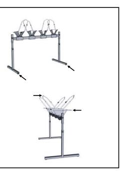
Use the provided Plugs to fill the exposed ends of the tubes.
