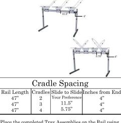
Place the completed Tray Assemblies on the Rail using our recommended spacing as directed in the chart above or according to your preference.
