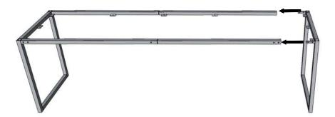
At each outer corner of the Frame Assembly (where the Corner Assemblies meet the Rails), insert two 5/16" x 3/4" Bolts with 5/16" Washers. Insert each bolt just until it catches. Then, tighten all bolts gradually in a rotating pattern until they are snug tightened. (Fully tighten in Step 4.)
