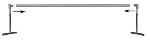
Next slide the ends of another Catch into the other end of the tray and loosely hold in place with a 1/4" Thumbscrew.
