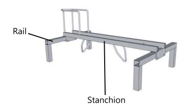
Step 2: Locate the Stanchion and insert  $1/2" \times 1"$  Black Plugs into the two open holes in the back and front of the Stanchion.
