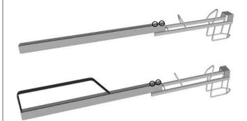
Locate the Stanchions and Trays. Flip a Stanchion and Tray upside down. Align the 2 holes in the Stanchion with the 2 holes in the Tray. The Tray should be on the outside of the Stanchion, as shown.
