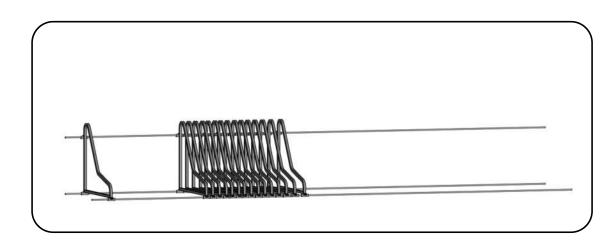
6. Space out your Side Frame placement by rolling the rear wheel of a bike between two Side Frames. Secure all Side Frames with (3) 1/4" x 3/8" Set Screws.
