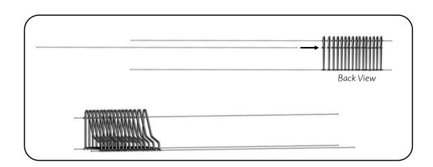
5. Loosen the previously secured Side Frame. Then set the End Side Frame with (3) 1/4" x 3/8" Set Screws.
