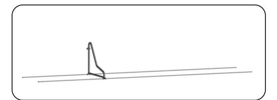
3. Repeat with the remaining Side Frames. Stack them at the end of the Runners, as shown.
