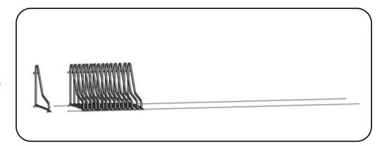
4. Slide the last Runner through the top tubes of the Side Frames.
